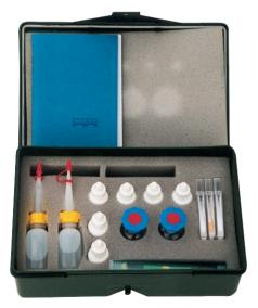
Allows the quick and easy assessment of the water quality. This kit lets anyone find out about the oxygen content, oxygen depletion value, pH value and temperature of the water as well as dissolved ammonium compounds.
