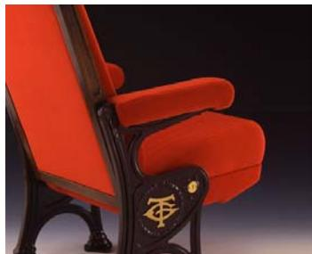
A special chair with classical lines. The seat comprises a metal structure and springs, a polyurethane foam block, upholstery, shell and hinge pins. The metal structure consists of two resistance-welded steel profiles forming a frame that holds a mesh of springs upon which the anatomically shaped cold-moulded polyurethane block rests.
