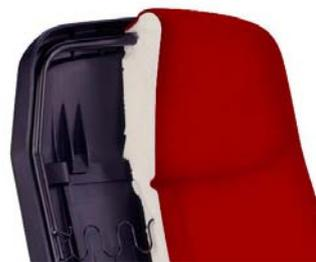
As the result of an exhaustive study, the seat's ergonomic design ensures that users enjoy maximum comfort. The seat and backrest are composed of two moulded polyurethane foam blocks with an interior metal structure. The upholstery is fully integrated into the foam by means of the INTEGRAL FORM system, without any hems or stitching.
