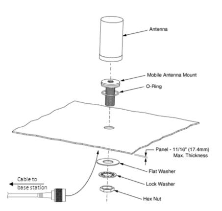
Figure 1: Remote Antenna Assembly
