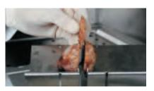
**3.** Raise the upper jaws and remove your 2 mm section from between the saw blades. The entire unit can be disassembled without tools for easy cleaning or disinfection.
