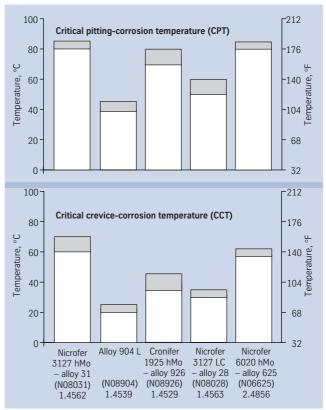
Fig. 7 – Critical pitting and crevice-corrosion temperatures of different alloys in 10% FeCl<sub>3</sub> x  $6H_2O$  solution.
