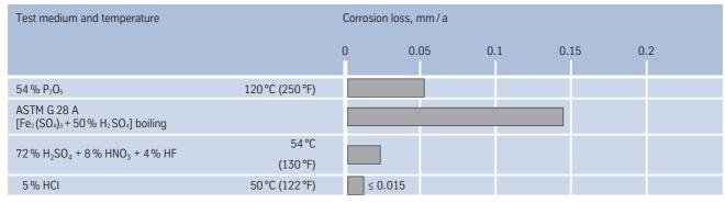
Fig. 8 – Corrosion loss of Nicrofer 3127 hMo in various media and at different temperatures.
