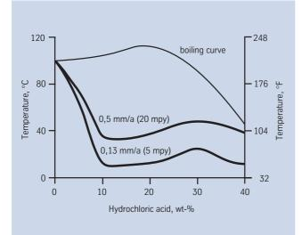
Fig. 9 – ISO-corrosion diagram of Nicrofer 3127 hMo in hydrochloric acid, determined in static immersion tests.
