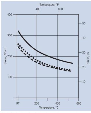
Comparison of typical short-time data for Nicrofer 3127 hMo – alloy 31 — with similar alloys as:
