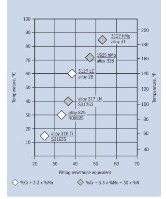
Fig. 6 – Critical pitting temperatures (CPT) in 10 % FeCl<sub>3</sub> x  $6H_2O$  solution as a function of the respective pitting resistance equivalents (PRE).
