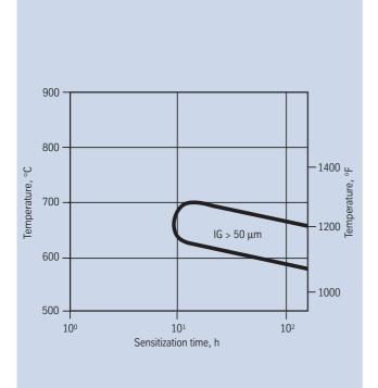
Fig. 4 – Time-temperature-sensitization diagram (TTS), IG according to the ASTM G 28 A test.
