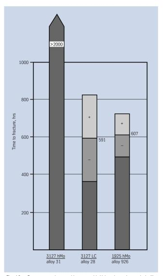
Fig. 10 - Stress corrosion cracking test with U-bend specimens in boiling 62 % CaCl<sub>2</sub>-solution.
