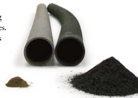
Comparison of APMT tube versus Fe-35Ni-25Cr after 2300 hours at 1100°C (2012°F). The FeNiCr tube is severely contaminated with oxide flakes.
