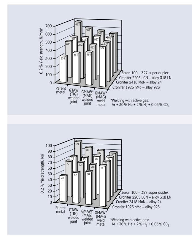
Fig. 1 - 0.2% Yield strengths at room temperature for weld joints of 6-Mo, high nitrogen austenitic, duplex and superduplex stainless steels with Nicrofer S 5020 – FM 50 filler metal.
