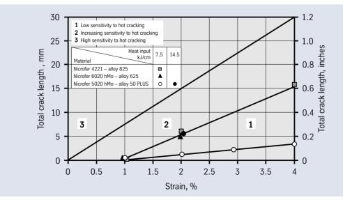
Fig. 4 - Hot cracking behaviour of Nicrofer 5020 hMo in comparison with Nicrofer 6020 hMo and Nicrofer 4221 in the Modified Varestraint Test (MVT).
