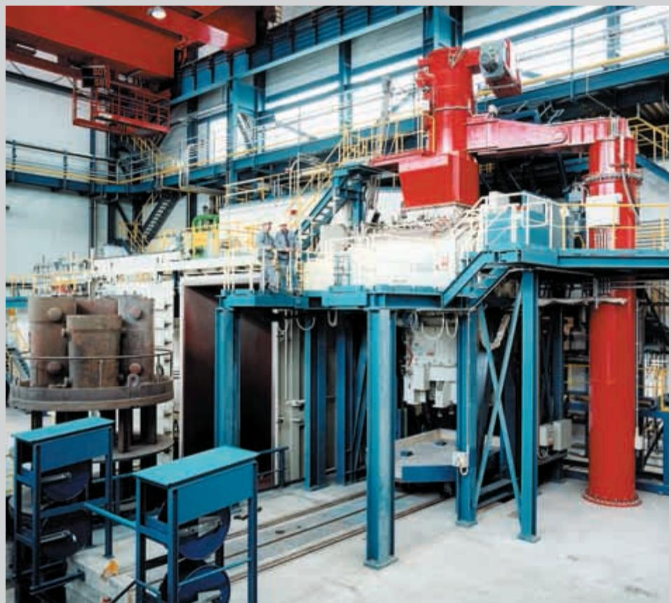
ThyssenKrupp VDM GmbH operates the world's largest VIM furnace, type VIDP, at its Unna melting plant.
