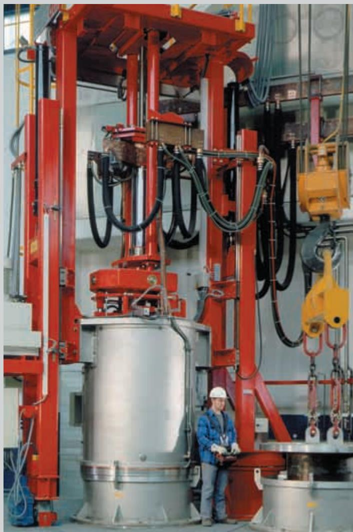
The new VAR-unit in the Unna melting shop is designed for ingot sizes up to 1,300 mm.
