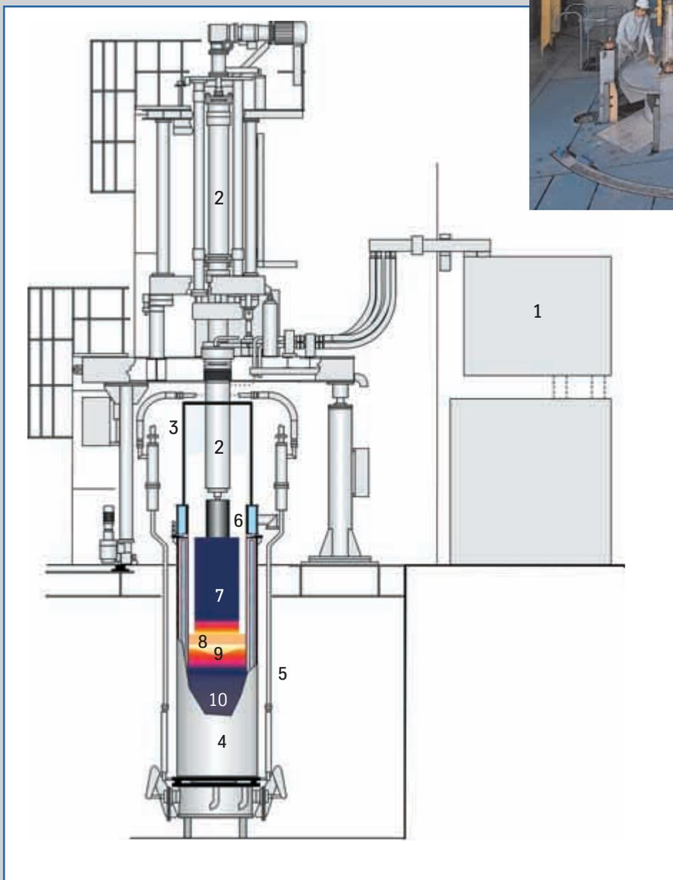
**New 20 tonne ESR-unit in the Unna melting shop. Upright mould with furnace lid enabling re-melting in protective gas atmosphere.**
