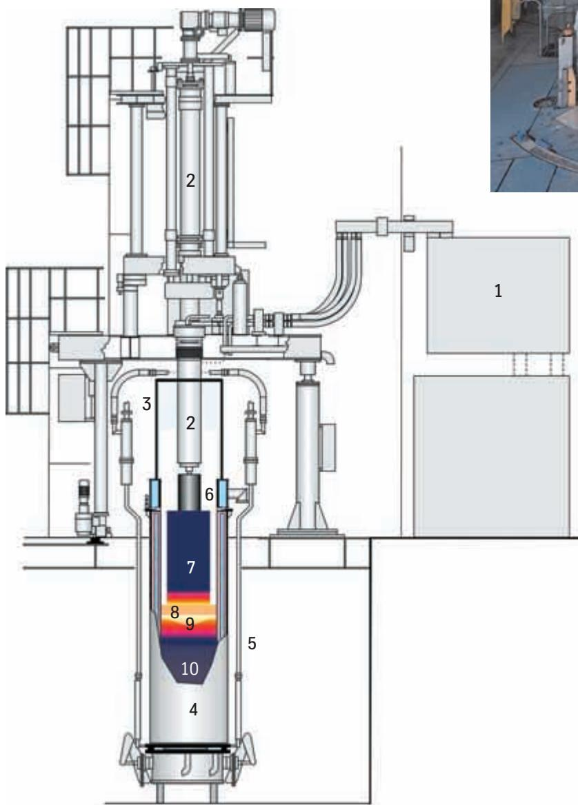
New 20 tonne ESR-unit in the Unna melting shop. Upright mould with furnace lid enabling re-melting in protective gas atmosphere.
