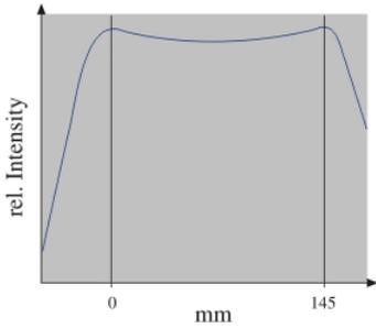
UV intensity in the longitudinal axis
