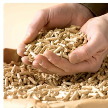
led combustion in a closed combustion chamber. Wood pellets can be burned in single stoves where the storage space must be regularly filled by hand; easier to handle are fully-automatic central heating units where the pellets are automatically transported by means of suction or a screw conveyor from a storage area to the burner.
