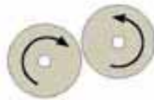
One Way and Uneven Directional Scrubbing of Conventional Disc Machines
