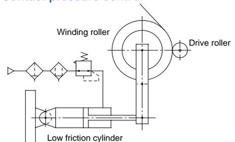
Pressure is kept steady, responding rapidly to the position change of a piston in the cylinder.
