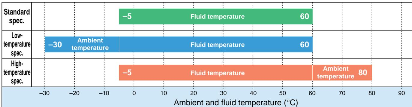
Note) The above indicates the temperature specification of a basic regulator for general purposes and a precision basic regulator. The standard temperature specification of an electronic regulator is ranging from 0 to 50°C.
