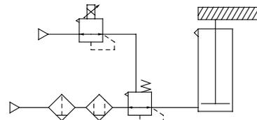
Pressure changes during cylinder actuation are suppressed, balancing the cylinder in both static and dynamic conditions.
