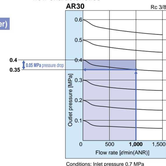
When the flow rate is 1,000 l/min (ANR) with the outlet pressure set to 0.4 MPa, the outlet pressure goes down (pressure drop) to 0.35 MPa due to the flow characteristics. The guideline of pressure drop should be set to less than 0.08 MPa against the set pressure; thus in this case the pressure drop is 0.05 MPa, which is within 0.08 MPa, so 0.35 MPa is within the tolerance.
