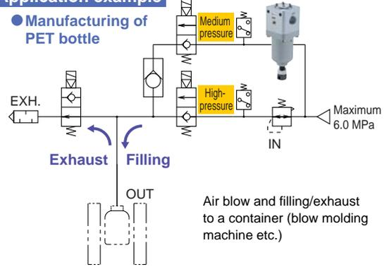
Air blow and filling/exhaust to a container (blow molding machine etc.)
