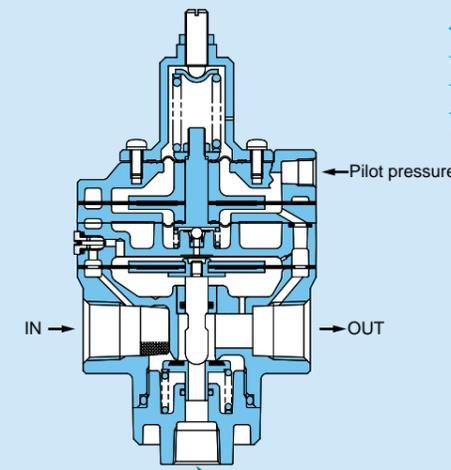
Relief port 3/8 Exhaust flow rate: Maximum 600 [ℓ/min (ANR)]
