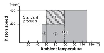
When using with the operating temperature fluctuated between 50°C or less and 100°C or more, the operating speed, etc. will be largely restricted by the durability. Prior to use, please contact SMC.
