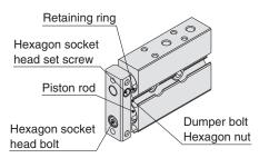
Note) The head cover retaining ring for ø6 is made of special steel.
