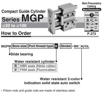
\* Iron parts made of stainless steel are available as made to order.
