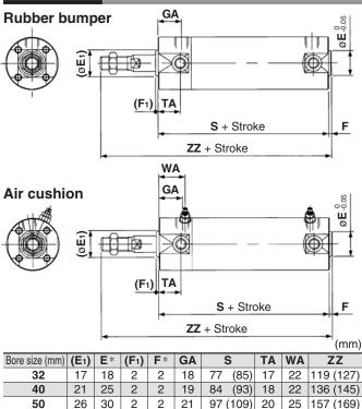
28 116 (130) 80 32 40 3 3 30 190 (204) 100 37 50 3 3 29 117 (131) 31 191 (205) Other specifications are the same as the double acting, single rod standard type. (An asterisk means it is the same as the standard type.) \* ( ): For the long stroke type.
