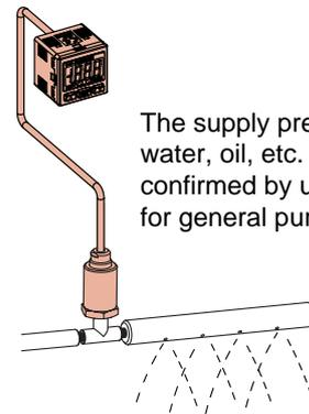
The supply pressure of water, oil, etc. can be confirmed by using a sensor for general purpose fluids.
