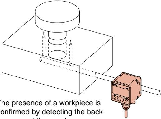
The presence of a workpiece is confirmed by detecting the back pressure at the nozzle.
