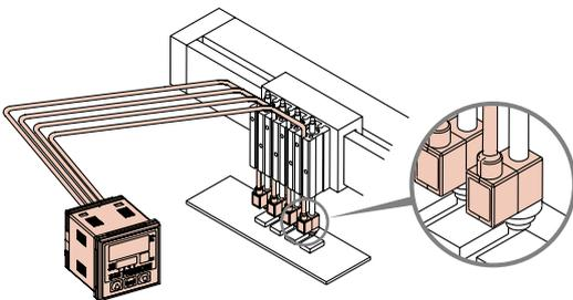
Due to the small size, the sensor can be installed close to a pad.
