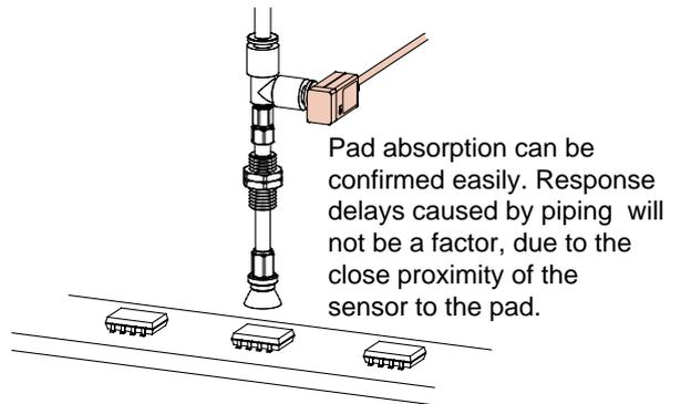
**Absorption confirmation of a workpiece absorbed with moisture**
