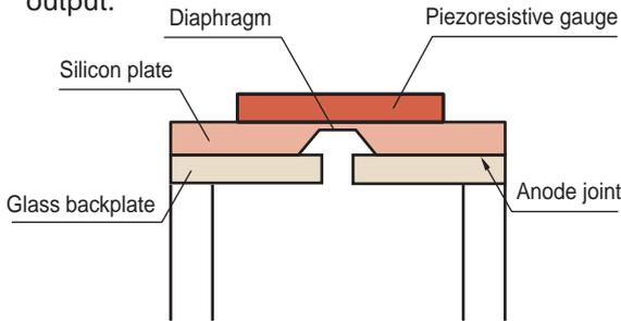
**Silicon diaphragm sensor construction**
