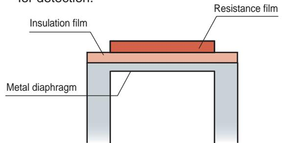
**Stainless steel diaphragm sensor construction**
