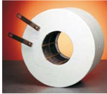
Fig. 2 RAC tubes with embedded but virtually free-radiating heating element, for a maximum element temperature of 1300°C (2370°F)
