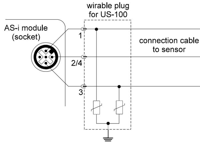
The varistors which can be mounted into a wirable plug prevent the occurrence of high electrostatic charges. One of these plugs per module is sufficient.
