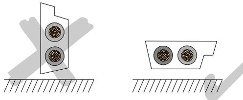
This also means the separate laying of the two AS-i cores which is absolutely to be avoided. A simple measure to improve symmetry to ground can be twisting the core ends or the twisted laying of the AS-i cable.
