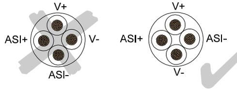
Twisting of the cable cores to compensate for the source of interference can, if possible, also be considered in this case as a measure to reduce interference. If this also proves to be insufficient, screening measures will have to be taken.
