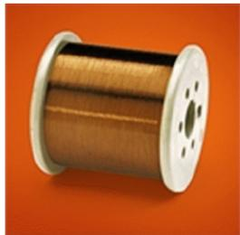
Round and flat conductive wire (magnet wire) in aluminium, copper-clad aluminium and copper. The Kanthal program includes standard conductive wire sizes but also custom-designed sizes and resistance to meet specific design requirements. The wire is available with or without insulation or coating.
