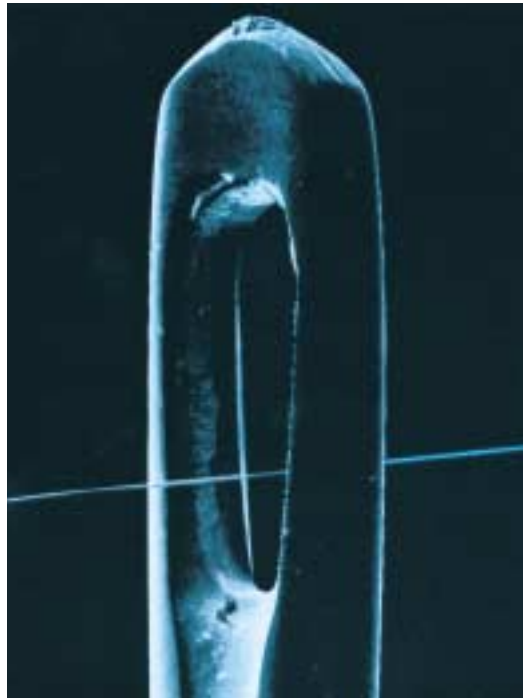
Precision wire 0.015 mm in the eye of a needle.
