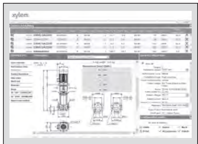
Dimensional drawings appear on the screen and can be downloaded in dxf format.
