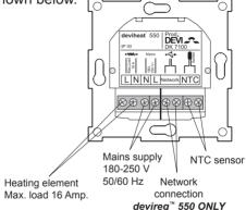
As the devireg<sup>™</sup> 540/550 is not equipped with an earth terminal, the earthing screen of the heating cable must be connected to the earth from the supply via the earthing terminal in the surface mounted box or the recessed metal box which ever is used.
