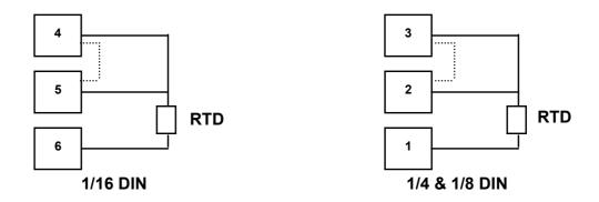
Figure 14 - RTD Input Connections
