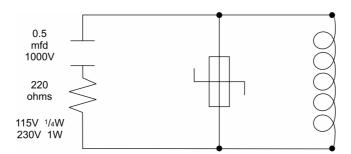
Figure 7 - Transient suppression with inductive coils
