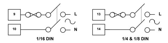
Figure 11 - Mains Power Connections
