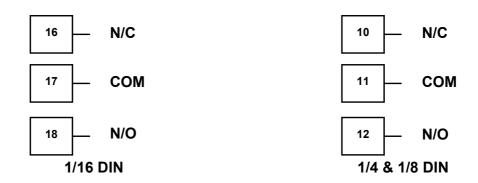
Figure 30 - Option Slot 3 - Relay Module
