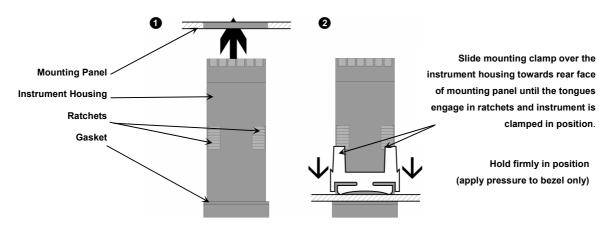
Figure 3 - Panel-Mounting the instrument
