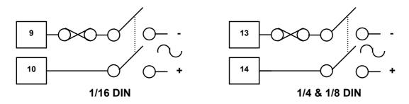
Figure 12 - 24/48V AC/DC Power Connections
