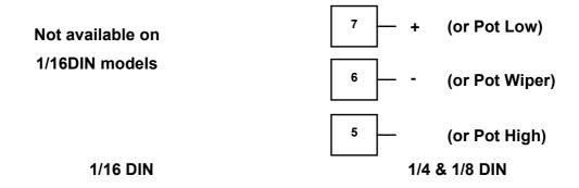
Figure 18 - Remote Setpoint Input Connections
