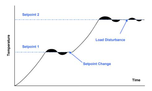
Figure 41 - Self-Tune Operation
