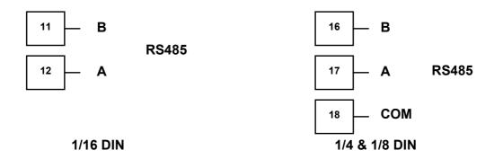
Figure 19 - Option Slot A - RS485 Serial Communications Module
