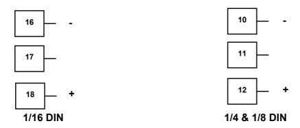
Figure 33 - Option Slot 3 - Transmitter Power Supply Module
