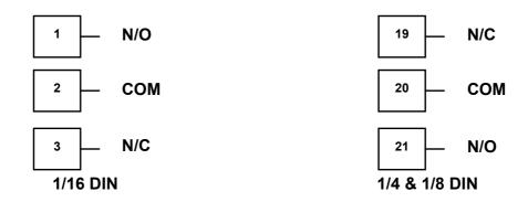
Figure 21 - Option Slot 1 - Relay Module
