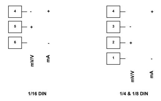
Figure 15 - DC Volt, mV & mA Input Connections
