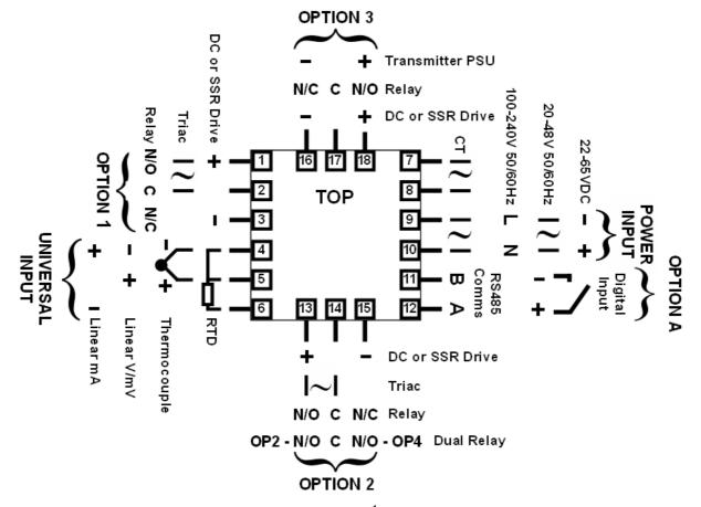
Figure 9 - Rear terminals (1/16-DIN Instruments)
