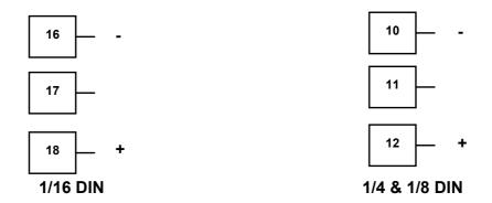
Figure 32 - Option Slot 3 - Linear Voltage or mADC module
