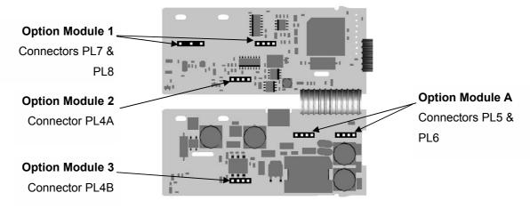
Figure 6 - Option Module Connectors
