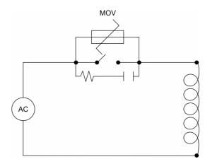
Figure 8 - Contact noise suppression
