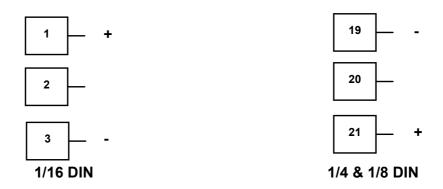
Figure 22 - Option Slot 1 - SSR Driver Module
