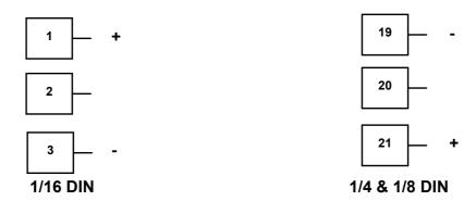
Figure 24 - Option Slot 1 - Linear Voltage or mADC Module
