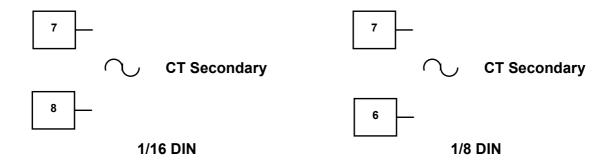
Figure 17 - Heater Current Input Connections
