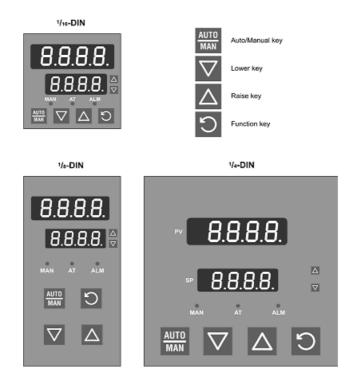
Figure 34 - Typical front panels
