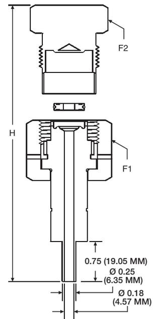
All Ultra High Integrity Pigtail Connections include nickel gasket
