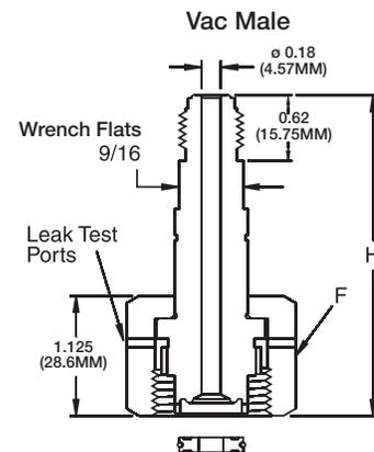
All Inlet Connections include nickel gasket 50-63-NI.
