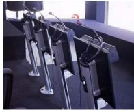
A beam-mounted, foldaway chair. The seat tips up, the back reverts to an upright position and the armrests fold up out of the way in a single, automatic movement. The seat tips up about its axis while the backrest moves forward until they are flat against one another.
