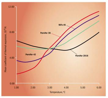
Fig. 1 - Coefficient of thermal expansion for Pernifer alloys
