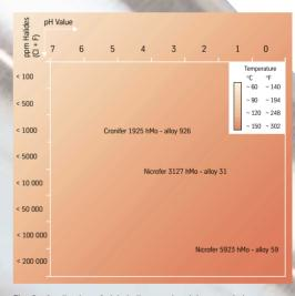
Fig. 2 - Application of nickel alloys and stainless steels in chloride (fluoride) contaminated acid (H<sub>2</sub> SO<sub>4</sub>)
