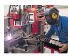
In the welding labortory at Altena, the base material's suitability for welding is examined, welding materials are developed and tested, and new processes are screened for their transferability to Krupp VDM high-performance materials.
