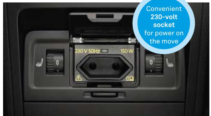
More and more European series-produced vehicle come with a 230-volt Euro socket. The required alternating voltage is generated by a WAECO inverter.
