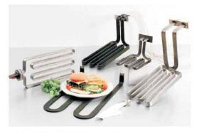
Reduced watt density - The surface area per linear inch of a Palenzo 1000 is 70 percent greater than the 0.430 inch (11 mm) diameter round tubular element. The Palenzo 625, is nearly 13 percent greater. This translates into longer heater life with optimum performance.
