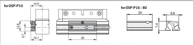
Note for OSP-P10: Switches can not be mounted directly opposite of the carrier !
