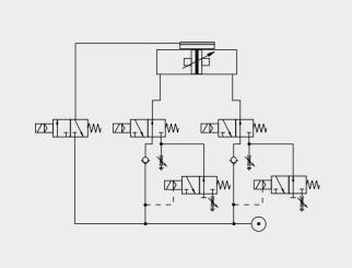
Fast/Slow speed cycle control with pneumatic brake for accurate positioning at high velocities.
