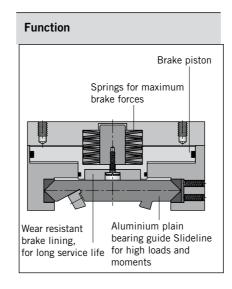
The high friction, wear resistant brake linings allow the Multi-Brake to be used as a dynamic brake to stop cylinder movement in the shortest possible time. The powerful springs also allow the Multi-Brake to be used effectively in positioning applications.
