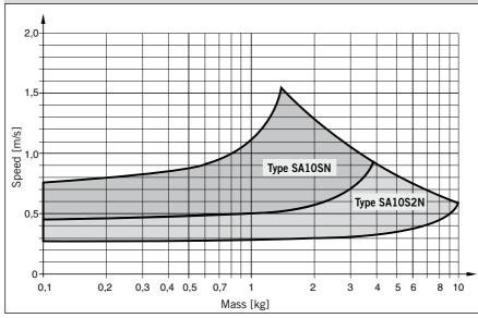
Shock Absorber Selection in Dependence on Mass and Speed for Series OSP-STL25
