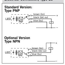
4 (Out) PIN assignment (view of pins) according to DIN EN 50044 1 (+) \* Length with possible minus tolerance, see chart below
