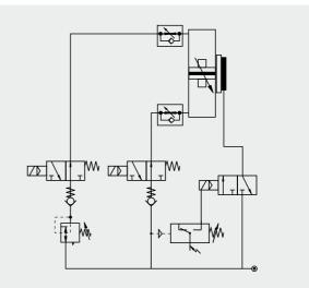
The combination of an OSP-cylinder with the passive MULTIBRAKE as shown here, allows accurate positioning and safety in case of loss of pneumatic air pressure. Examples
