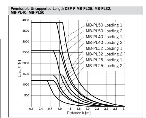
Mid section supports are required from a certain stroke length to prevent excessive deflection and vibration of the linear drive. The diagrams show the maximum permissible unsupported length in relation to loading. A distinction must be drawn between loading 1 and loading 2. Deflection of 0.5 mm max. between supports is permissible.
