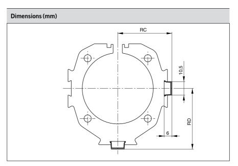
For clean guidance of magnetic switch cables along the cylinder body. Contains a maximum of 3 cables with diameter 3 mm. Material: Plastic Colour: Red Temperature Range: -10 to +80 °C
