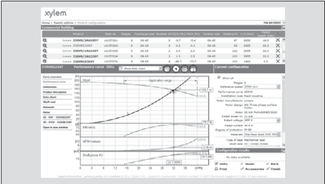
The detailed output makes it easy to select the optimal pump from the given alternatives.
