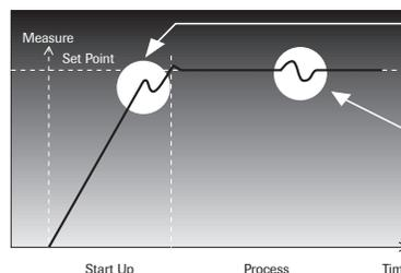
**During Start-Up** the SMART self-tuning function calculates the control parameters to optimize the rise to set-point.
