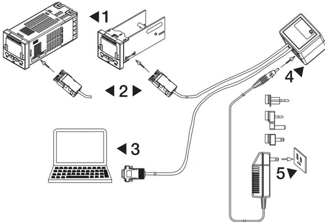
The 1601E can be connected to the remote Configuration Kit, CNFG-10000. This method of configuration is ideal for OEM's for quick setup and for resellers to easily program a controller for the specific needs of a customer.
