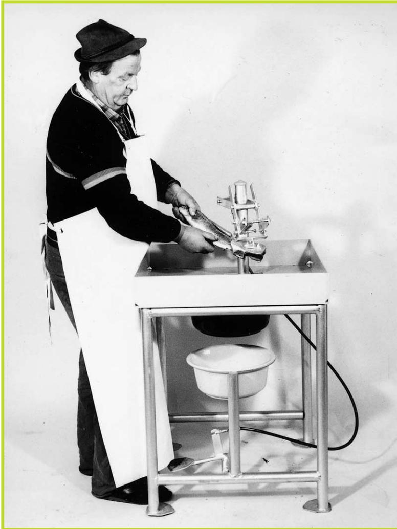
Fish can be stripped of their eggs very gently and professionally using the AGK roe stripper. The fish cannot hurt itself as it wiggles for freedom – it is securely pinched by the machine. Thus the whole procedure will not be overly prolonged.
