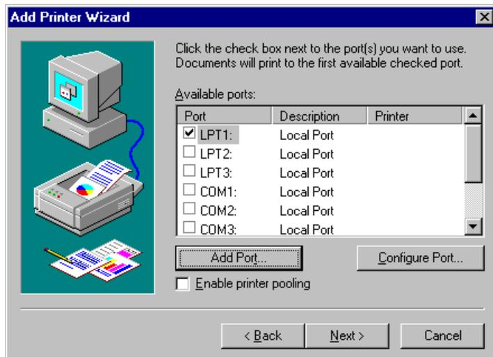
Click the **Add Port** button and select from the next window **CV TCP/IP Monitor** from the list of **Available Printer Ports**.
