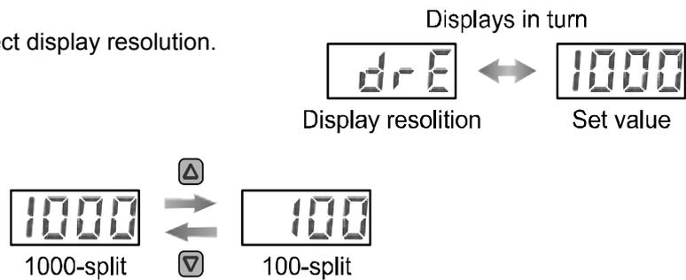
Press the  $\text{\$}$  button to set.  $\downarrow$  Return to function selection mode.
