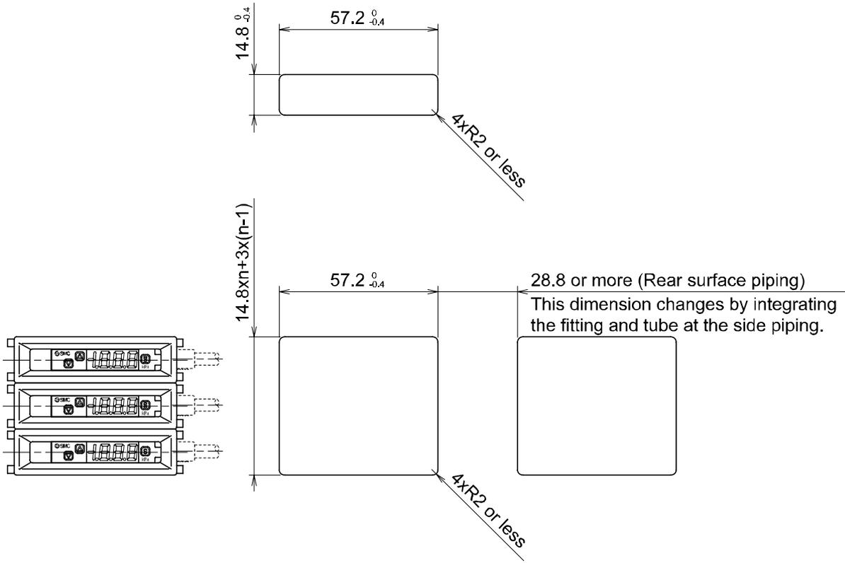
○DIN rail mounted side piping
