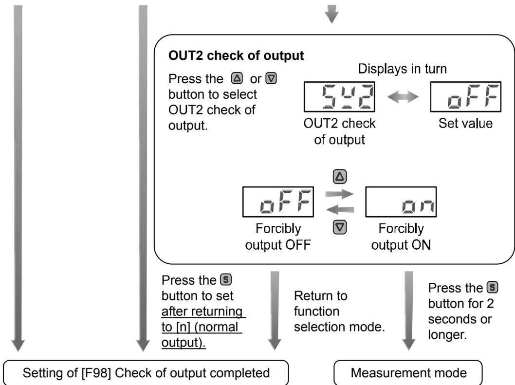
\*: If the  $\Delta$  button is pressed for 2 seconds or longer, the mode is returned to measurement mode regardless of the current mode.
