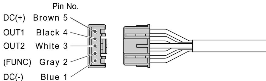
■ Internal circuit and wiring example
