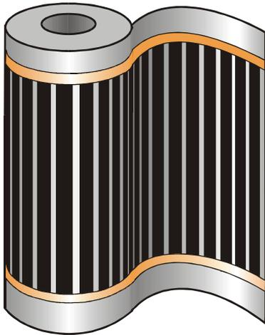
**Flexel** consists of a specially formulated semi-conductive medium, coated onto polyester film. Power is fed to this resistive coating by way of copper electrodes that are fixed to the longitudinal edges of the heating areas. This structure is insulated by a lamination of polyester based films that totally cover the element and is wider than the conductive heating area, forming strong clear edges that are designed to accept subsequent stapling to ceiling joists.
