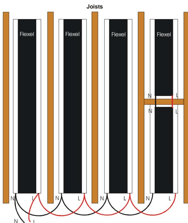
In certain cases where access to the ceiling is available, **Flexel** elements can be installed from above. Where cross noggins, light fittings or other obstructions occur, the element must be bridged as shown, in the illustration on the left. A minimum 150mm space either side of any obstruction must be maintained.
