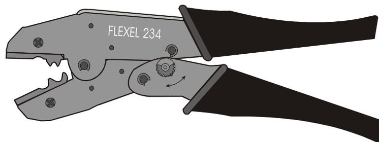
1. Remove the retaining ring or the locking screw from the eccentric axle.
