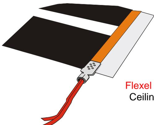
Using the recommended "**Flexel 234**" pliers complete the crimp connection with the tool so that the "W" form of the tool is to the seamed side of the cylindrical ferrule of the crimp. If crimped in reverse the crimp cover may not fit.
