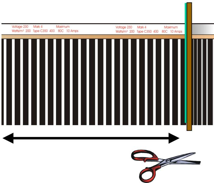
Unroll the element on a clean working surface and check for any damage.
