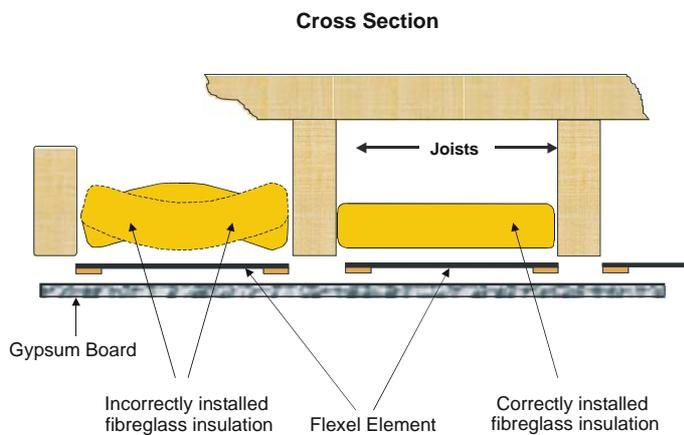
In some instances, insulation can be installed after the **Flexel** elements have been fixed, for example in the roof space in bungalow type constructions or pitched roof two storey dwellings.
