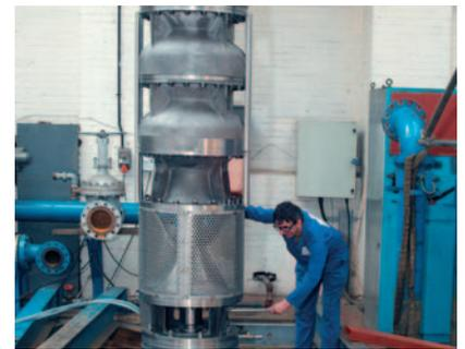
Designed to complement the **Hayward Tyler** motor range, our submersible solutions offer a comprehensive choice for the materials of construction. The pump duty is matched to customer requirements by selecting the pump size, number of stages and trimming the impellers. The applications are usually seawater lift or firewater pumps. The pumps are supplied, fitted to and powered by a submersible motor.
