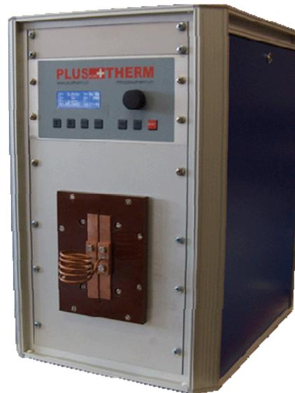
**TNX 5-20 Compact with external resonance circuit**
