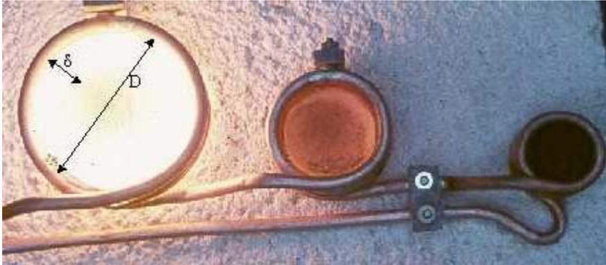
Three inductors are connected in line (equal current for every coil). The equation  $D > 2 \times \delta$  is only valid for the first coil (left side). The work piece in the last coil (right side) is not heated, because  $D < 2 \times \delta$ .
