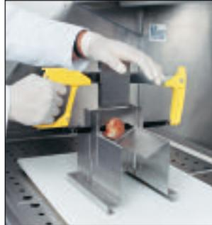
Raise the upper jaws and remove your 2 mm section from between the saw blades. The entire unit disassembles without tools for easy cleaning or disinfection.
