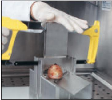
Raise the upper jaws and remove your 2 mm section from between the saw blades. The entire unit disassembles without tools for easy cleaning or disinfection.
