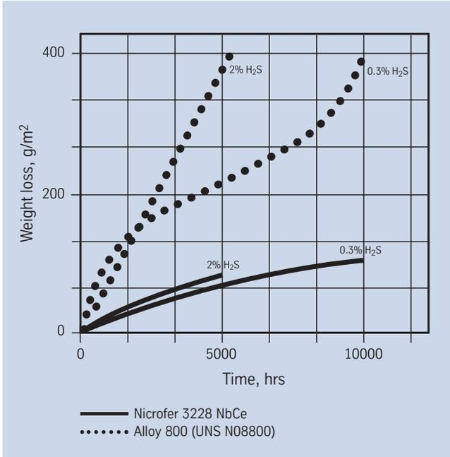
Fig. 7 – Comparison of weight loss of Nicrofer 3228 NbCe and alloy 800 respectively in high- and low-sulfur containing process gases at 940 °C (1724 °F) after 10,000 hrs.
