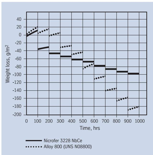
Fig. 3 – Effect of cerium content (< 0.1%) on the weight loss of austenitic Fe-Ni-Cr alloys under thermal cyclic conditions involving 10 cycles of 100 hrs each at 1050 °C (1922 °F) followed by cooling to room temperature.
