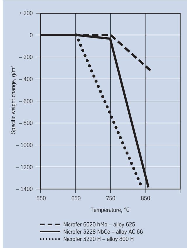
Fig. 9 – Influence of temperature on behaviour in a typical waste incineration atmosphere under cyclic conditions: Comparison of specific weight change in a simulated waste incineration environment consisting of nitrogen with 9% O<sub>2</sub>, 2.5 g/m<sup>3</sup> HCl and 1.3 g/m<sup>3</sup> SO<sub>2</sub> after 1000 hrs cyclic exposure at temperatures of 550 to 850 °C (1022 to 1562 °F).
