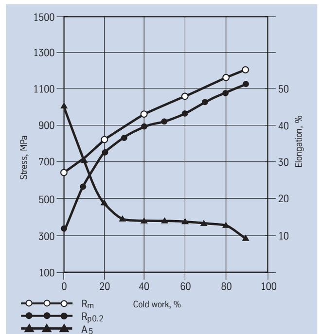
Fig. 2 – Effect of cold work on the mechanical properties of Nicrofer 3228 NbCe.
