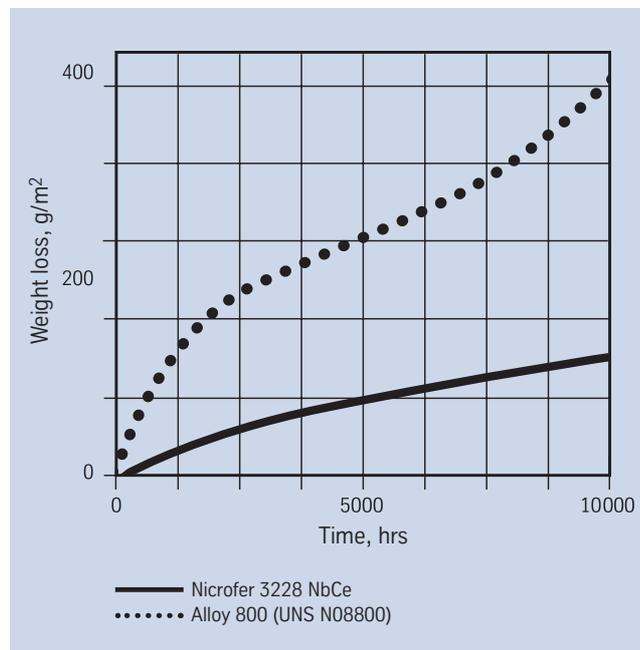
Fig. 4 – Weight loss comparison in air at 980 °C (1796 °F) during 10,000 hrs simulating oxidation behaviour under oxidizing conditions at high temperature of Nicrofer 3228 NbCe with alloy 800.
