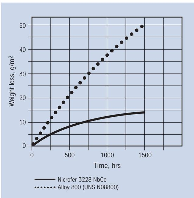
Fig. 8 – Comparison of weight loss of Nicrofer 3228 NbCe and alloy 800 in an H<sub>2</sub>/H<sub>2</sub>O/HCl atmosphere at 900 °C (1652 °F) after 1500 hrs.
