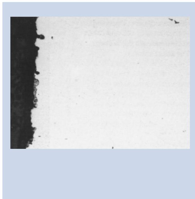
Fig. 6 – Nicrofer 3228 NbCe without evidence of internal oxidation in an oxidizing atmosphere at 980 °C (1796 °F) after 10,000 hrs.
