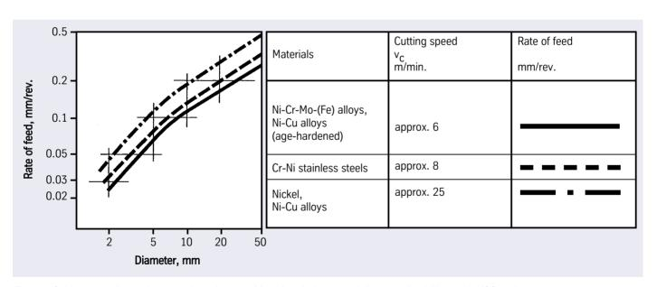
Fig. 5 – Guide values for cutting speeds and rates of feed in relation to tool diameter for drilling with HSS tools
