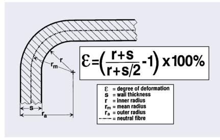
Fig. 1 – Calculation of the degree of cold deformation in bending
