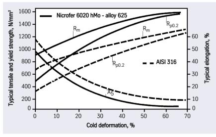
Fig. 2 – Effect of cold deformation on mechanical properties
