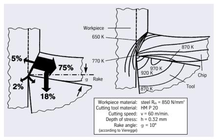
Fig. 4 – Heat distribution in the workpiece, chip and tool during machining of steel according to Kronenberg
