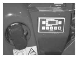
6. Electric motor regulates by-pass when using the optional computer system
