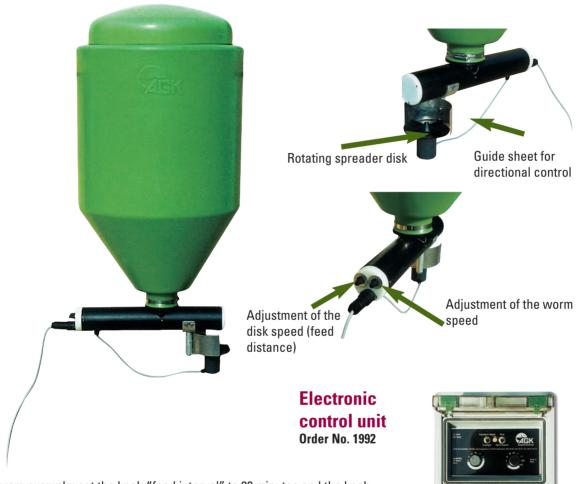
Program example: set the knob "feed interval" to 32 minutes and the knob 'quantity of feed" to 4 seconds, then the dispenser will feed every 32 minutes for the time of 4 seconds.
