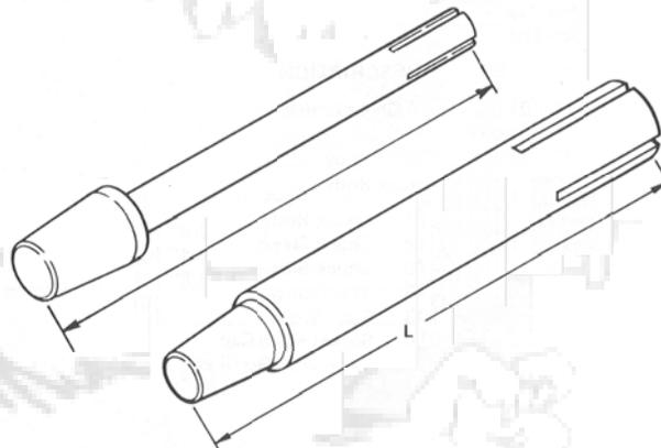
4-3/4" Long Length Fixed Chuck Depth (1/2") Chucks
