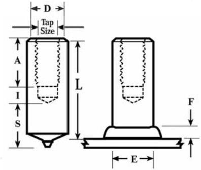
When ordering, specify **Type**, **Diameter**, **Before Weld Length**, **Tap Size**, **Material**, **Quantity**, and **Part Number**
