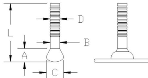
The flat top caps for use with N3A studs are usually supplied in aluminum. They can also be supplied in plated mild steel or stainless steel, per the N3P Annular Ring stud.
