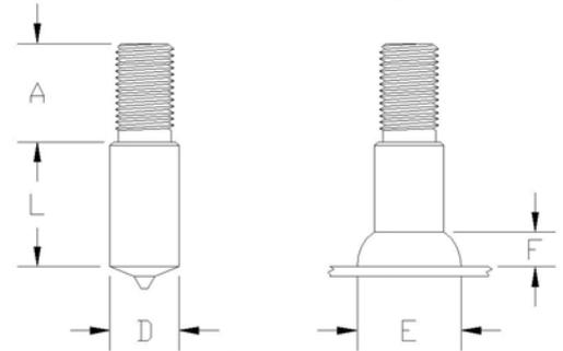
**When ordering, specify Type, Base Diameter, Base Length, Extension Thread Size, Extension Length, Material, Quantity, and Part Number**
