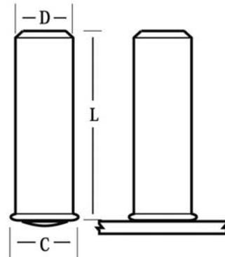
Nelson Stored Arc studs have a flanged weld base that is about 1/32", or 1mm, greater than the nominal stud diameter. The "A" flange allows automatic stud feeding for increased production speeds. The flange also increases the stress area on the sheet. Standard studs come in lengths up to 1.25".
