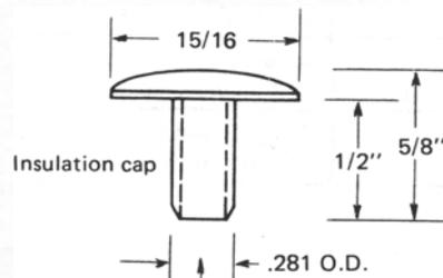
**Materials:** The Navy pin cap is supplied in Aluminum. For specific grade information and physical and chemical properties, and conforming standards, please see [General Material Specifications](#).
