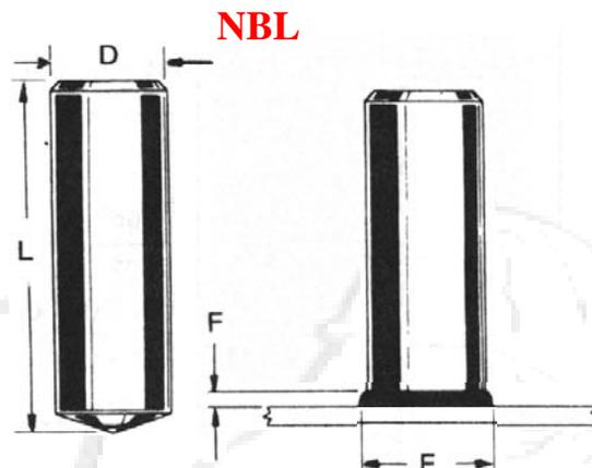
**When ordering, specify Type, Diameter, Before Weld Length, Material, Quantity, and Part Number**
