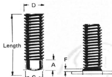
When ordering, specify **Type, Diameter, Before Weld Length, Material, Quantity, and Part Number**
