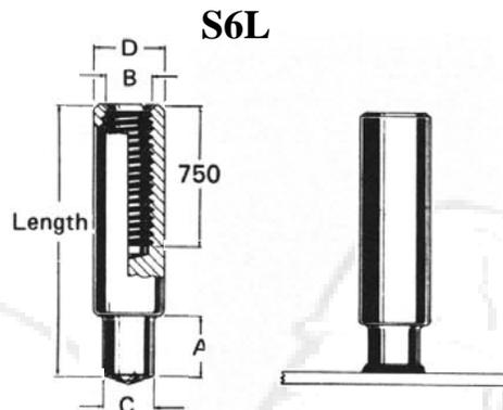
When ordering, specify Type, Diameter, Before Weld Length, Material, Quantity, and Part Number
