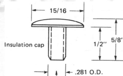
**Materials:** The Navy pin cap is supplied in Aluminum. For specific grade information and physical and chemical properties, and conforming standards, please see [General Material Specifications](#).
