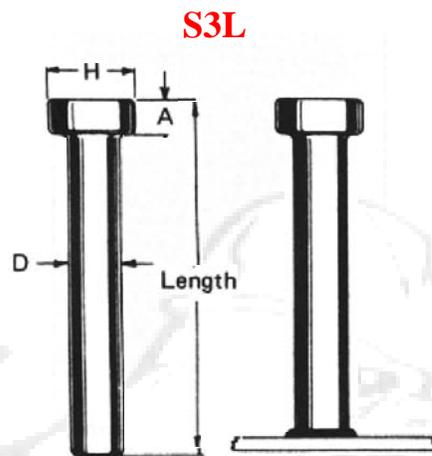
Shear connectors are typically used in composite steel construction for holding concrete slabs to steel members to resist shear forces and increase shear loading capacity in steel buildings, bridges, columns caissons, containment liners, etc. They also act as embedment anchors on miscellaneous embedded plates, frames, angles, strip plates, attachments and connections. Options for **Welding Through Metal Deck** are available for this stud.
