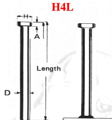
**When ordering, specify Type, Diameter, Before Weld Length, Material, Quantity, and Part Number**
