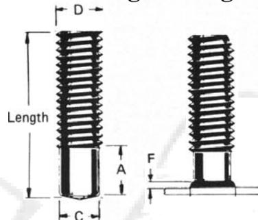
**When ordering, specify Type, Diameter, Before Weld Length, Material, Quantity, and Part Number**
