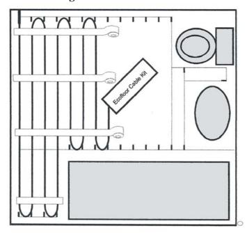
Connection is only required at one end. The first 3metres is black cable that can be cut as required. The orange cable is the heated part that must never be cut or shortened.
