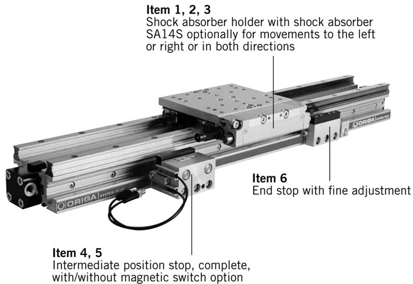
Illustration shows version with shock absorber holder for movement in both directions and magnetic switch option with T-slot switches (for magnetic switches Accessories see from page 123)
