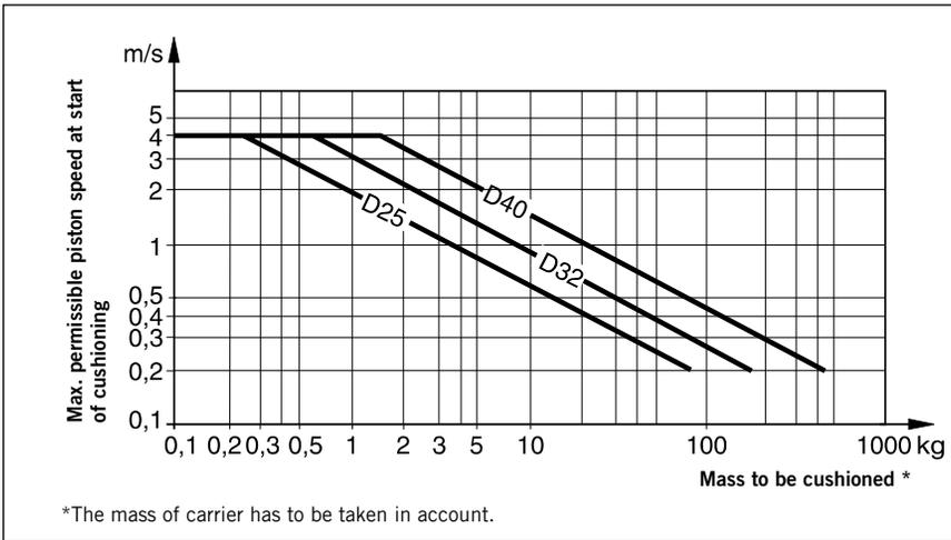
**If the permitted limit values are exceeded, additional shock absorbers should be fitted in the area of the centre of gravity.**
