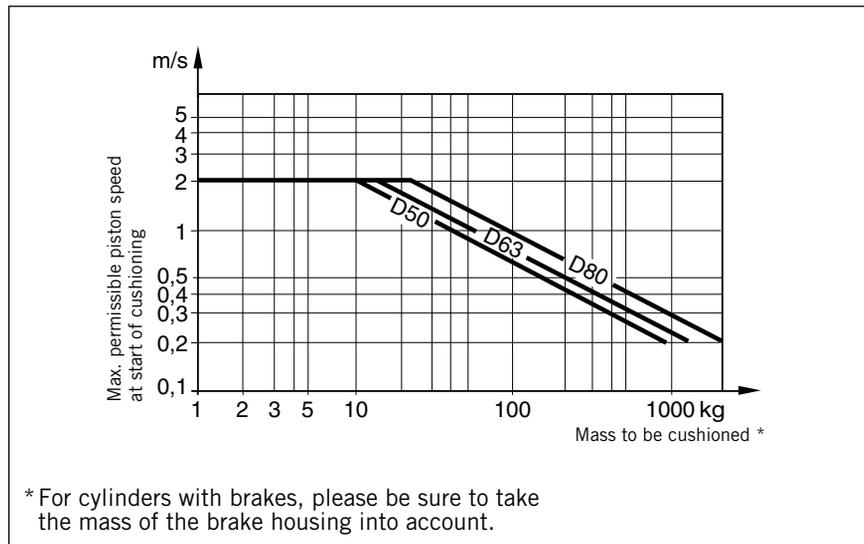
**If the permitted limit values are exceeded, additional shock absorbers should be fitted in the area of the centre of gravity .**
