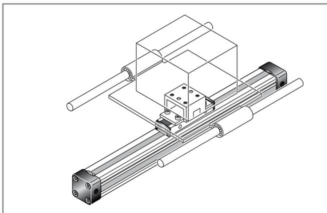
When using external guides, the clevis mounting is used to compensate for deviations in parallelism.
