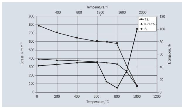
Fig. 1 – Typical short-time properties of solution-treated Nicrofer 7016 TiAl rod and bar products at room and elevated temperatures.
