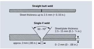
Fig. 3 – Edge preparation for welding of nickel alloys and special stainless steels.
