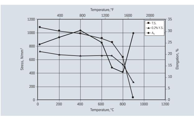
Fig. 2 – Typical short-time properties of solution-treated and age-hardened Nicrofer 7016 TiAl rod and bar products at room and elevated temperatures.
