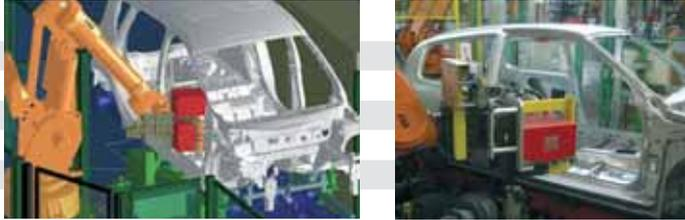
Fully automated robot-based marking
