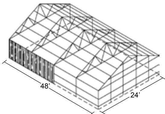
This greenhouse is engineered to meet 70 mph wind and 10 pound live load per the UBC Building Code. Higher load ratings and stamped engineered plans are available at extra cost. All galvanized steel frame insures maximum strength and life. Lexan twin-wall polycarbonate covering is UV resistant with a 10 year discoloration warranty.
