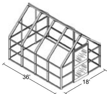
This greenhouse is engineered to meet 70 mph wind and 10 pound live load per the UBC Building Code. Higher load ratings and stamped engineered plans are available at extra cost. All galvanized steel frame insures maximum strength and life. Lexan twin-wall polycarbonate covering is UV resistant with a 10 year discoloration warranty.
