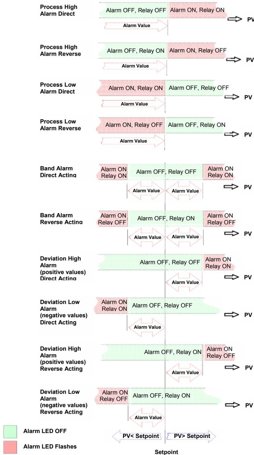
Figure 38 - Alarm Operation
