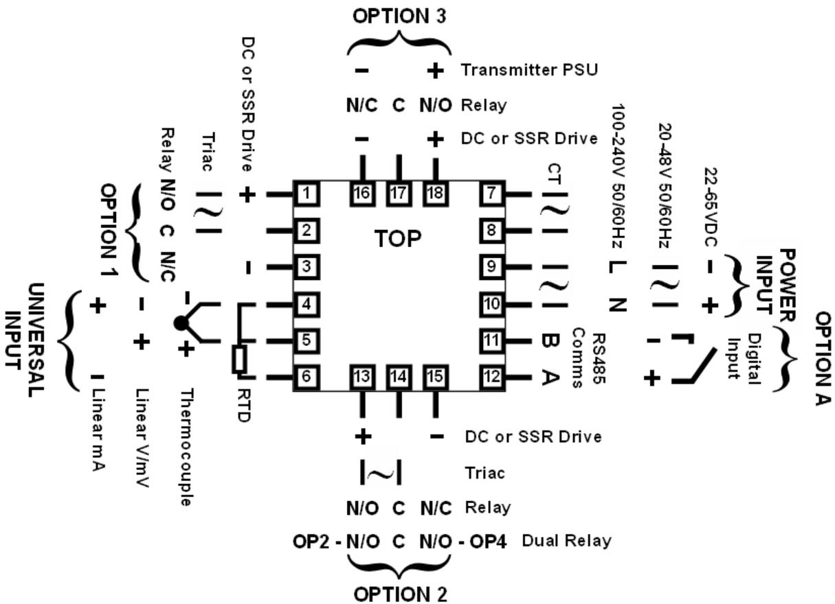
Figure 9 - Rear terminals ( $1/16$ -DIN Instruments)
