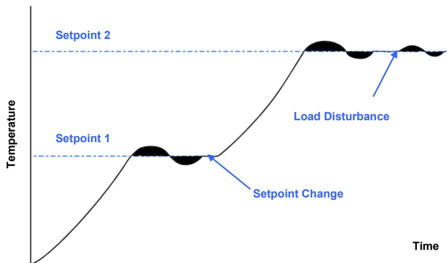
Figure 41 - Self-Tune Operation
