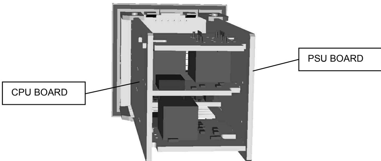
Figure 4 - Typical rear view (uncased) showing PCBs positions
