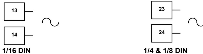
Figure 28 - Option Slot 2 - Triac Module
