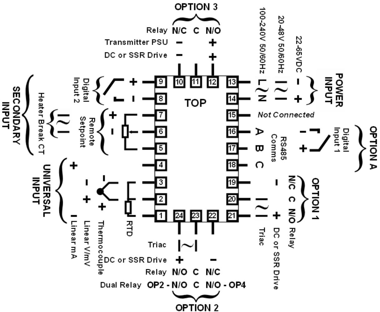
Figure 10 - Rear terminals (1/4-DIN & 1/8-DIN Instruments)
