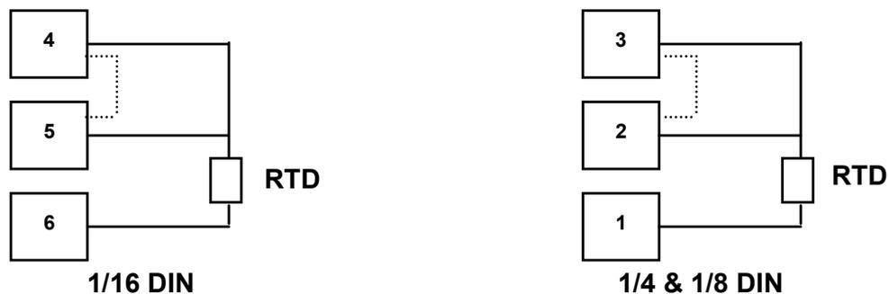
Figure 14 - RTD Input Connections
