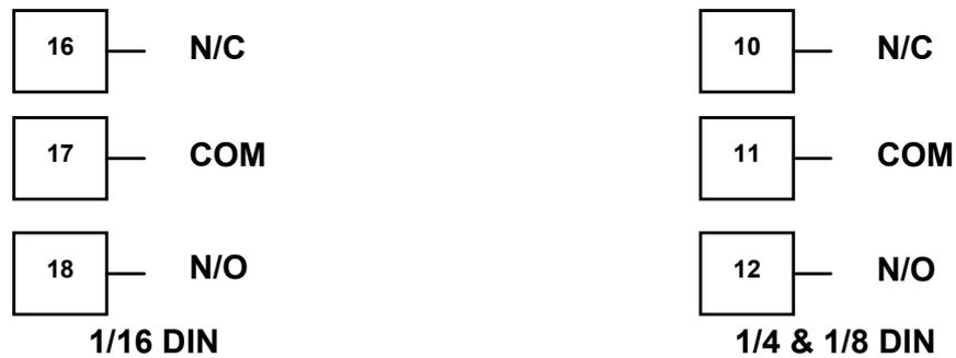
Figure 30 - Option Slot 3 - Relay Module
