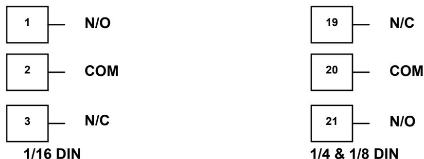
Figure 21 - Option Slot 1 - Relay Module
