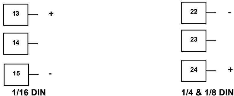
Figure 29 - Option Slot 2 - Linear Voltage or mADC module
