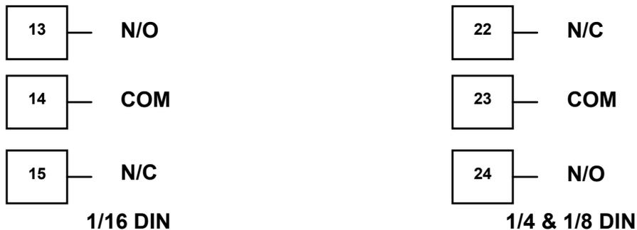
Figure 25 - Option Slot 2 - Relay Module
