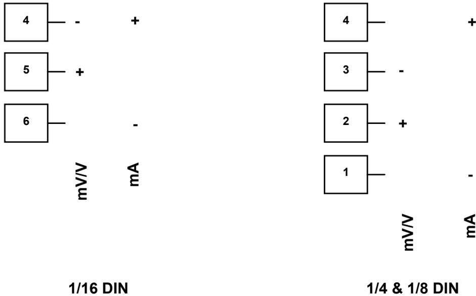
Figure 15 - DC Volt, mV & mA Input Connections
