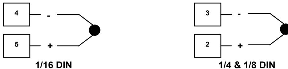
Figure 13 - Thermocouple Input Connections
