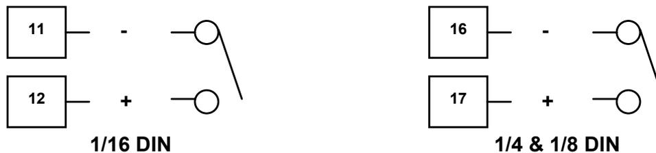
Figure 20 - Option Slot A – Digital Input Module
