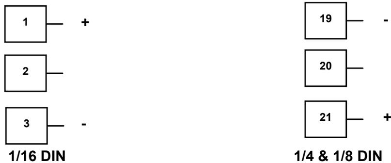
Figure 24 - Option Slot 1 - Linear Voltage or mADC Module
