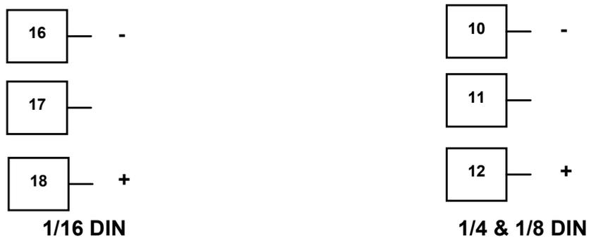
Figure 31 - Option Slot 3 - SSR Driver Module
