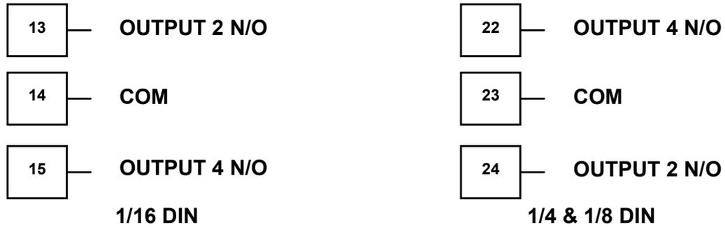
Figure 26 - Option Slot 2 - Dual Relay Module
