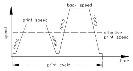
In case of 'time critical' applications you have the possibility with a good selection of different device parameters to increase the effective print speed and it this way the clock cycle.
