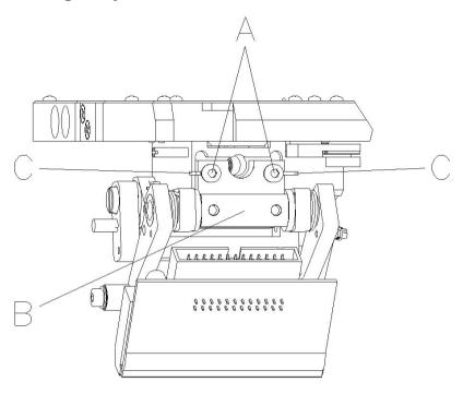
The installation angle of the printhead is default 26° to the print surface. However, manufacturing tolerances of printhead and mechanics can require another angle.
