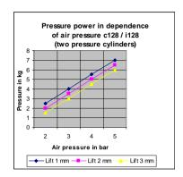
The pressure power of the printhead can be set with the pressure regulator. The values are indicated in the following table:
