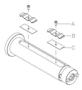
If other transfer ribbons are used, it can occur that the clamping force of the spring plates (B) is not sufficient, in order to position the rolls surely and to protect it against rotating.
