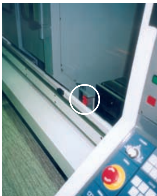
Example of use: TZK use on sliding doors of tool machines
